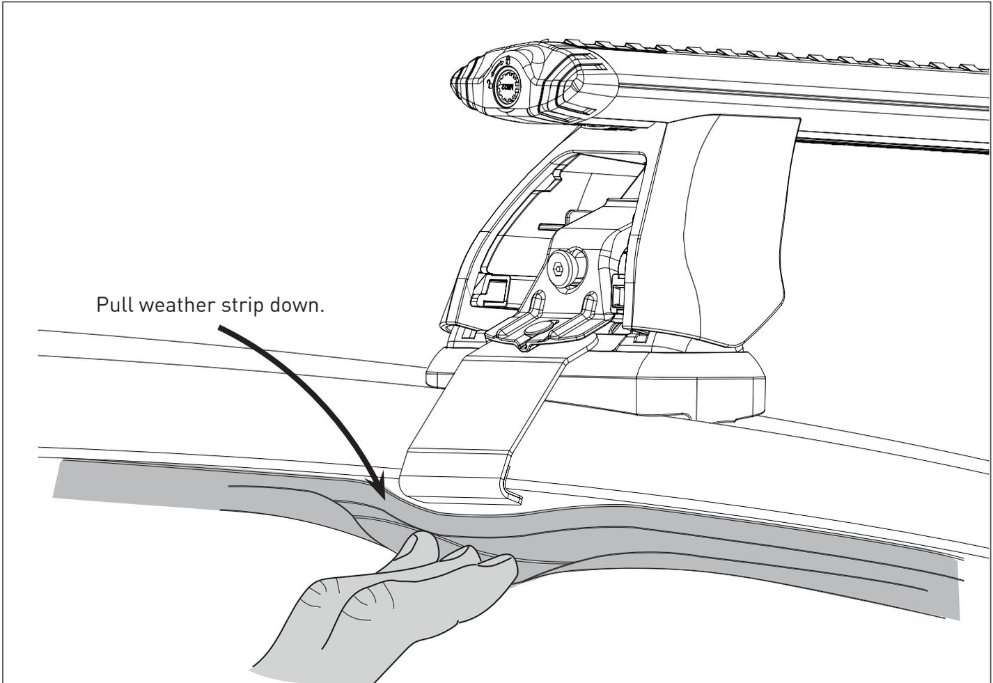
With doors open, gently pull the top weather strip down. Fit the two piece bracket assembly so the lower bracket sits above the rubber and hooks the radius of the vehicle roof. Fit the M8 attachment screw. Repeat for each side, front & rear of vehicle.
